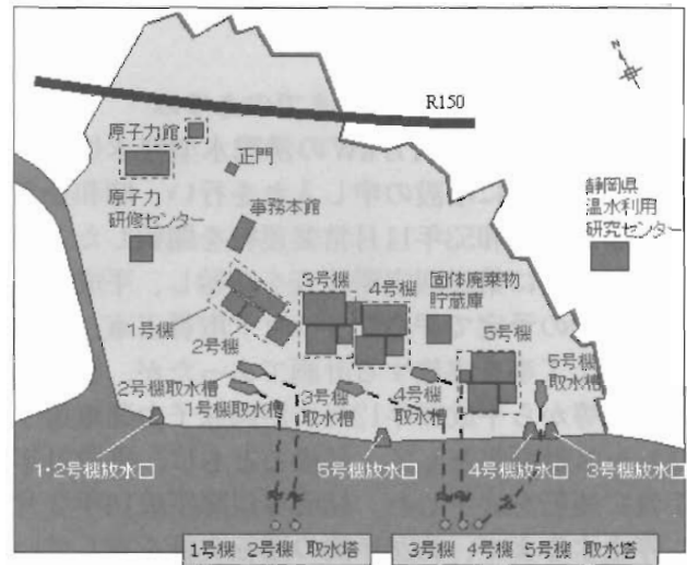
Fig.2 Main Equipment Arrangement
