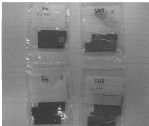
Fig.10 Mock Contaminated-materials of the Primary Cooling System in the Nuclear Power Reactor.
